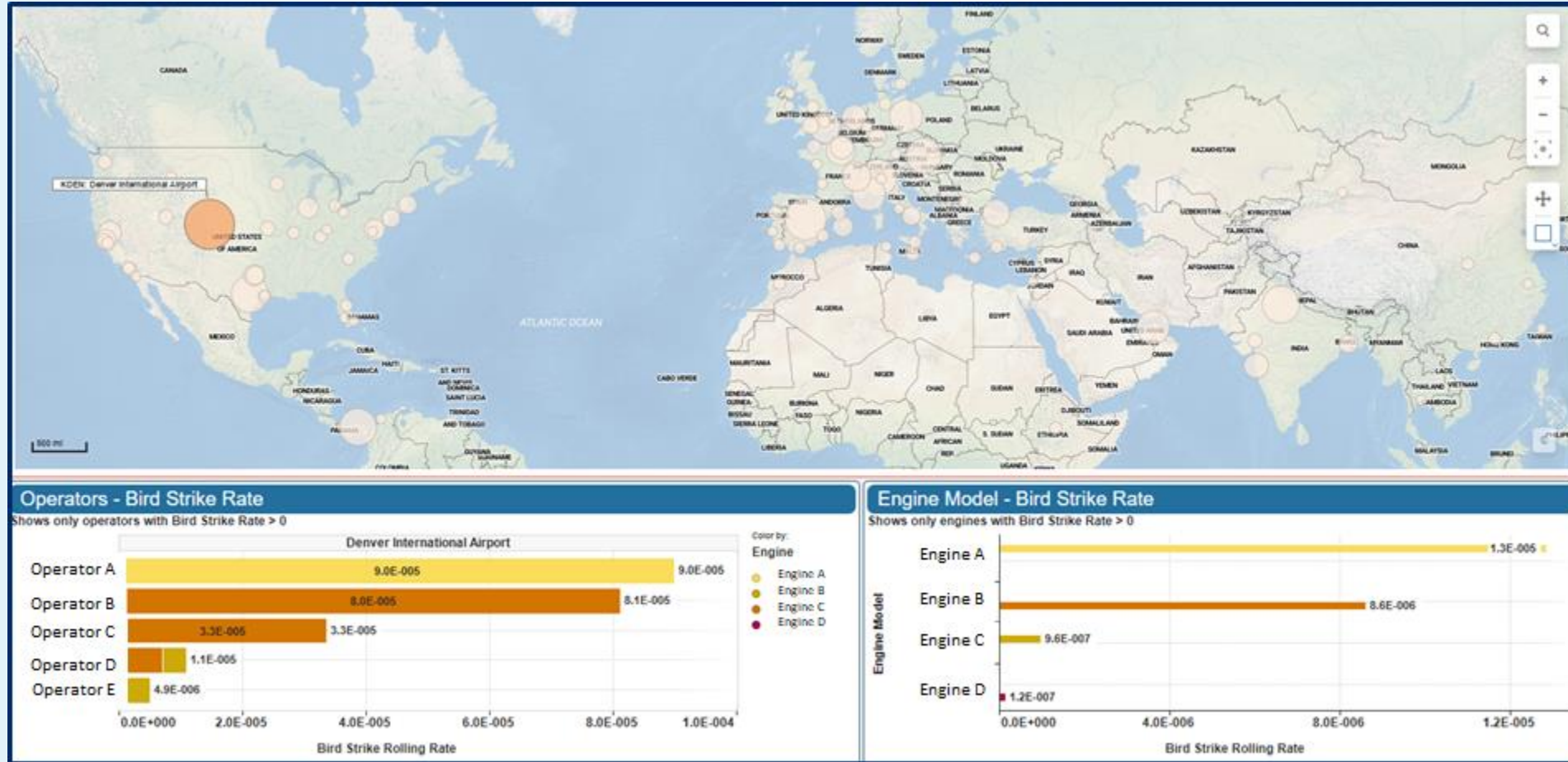
Bird Engine Strike Events by Airport– GE/CFM Commercial Engines Only (2023 event data)
