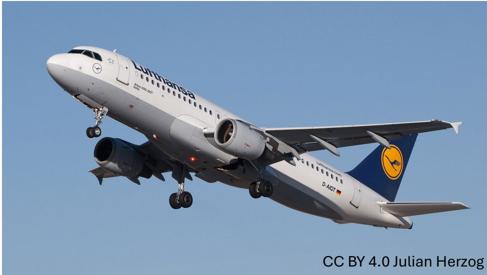
Airbus A320 – fuselage diameter 3.95 m
